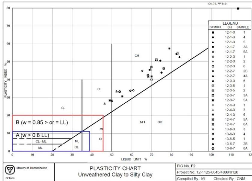
Figure 4. Type of soils which could be liquefiable showing that the soil at the landfill site are not susceptible to ‘classic’ liquefaction according to Seed et al. (2003). Zone A: below the blue line; Zone B: above the blue line and below the red line. In all cases, the water content has to be close to or above the liquid limit. The Leda clays tested at the Boundary Road site all fall outside regions A and B.
