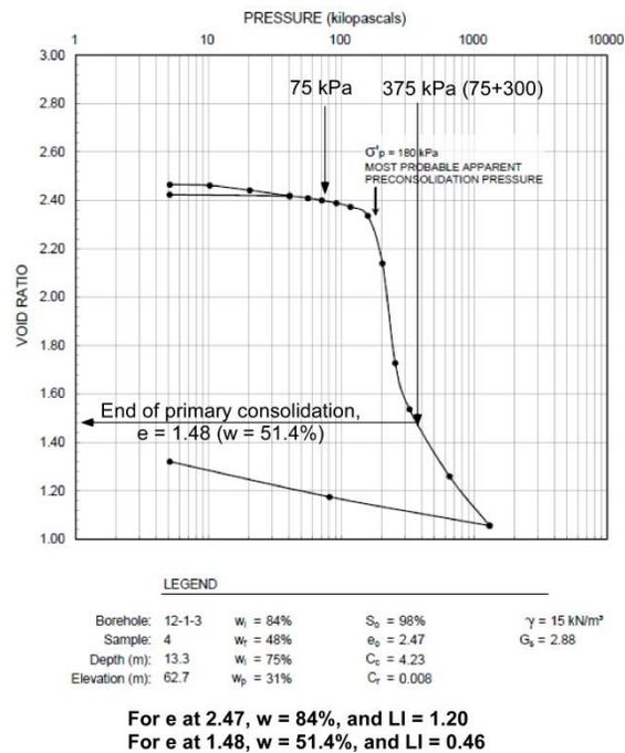
Figure 3. Estimation of changes in void ratio and water content at the end of primary consolidation for a sample located at a depth of 13.3 m.
