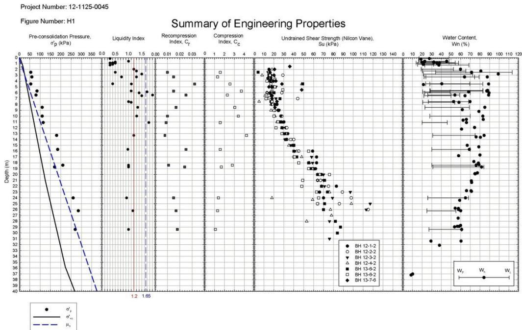
Figure 1. Modified geotechnical profile found in Appendix H, Figure H1 providing the actual data on the liquidity index and specific lines for values of 1.2 and 1.65.
