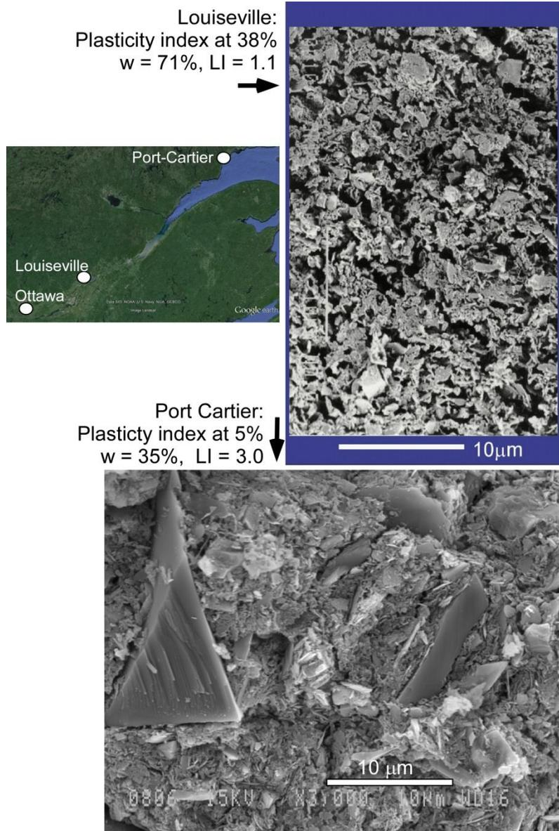
Figure 2. Microphotographs of marine sediments at Louiseville and Port-Cartier shown at about the same scale (white bar at 10 microns). Note the very great difference in the grain size of both samples, the Port-Cartier sample being much coarser (see the triangular quartz grain to the left) than the Louiseville sample. [w = water content; LI = liquidity index]
